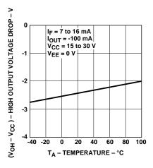
Figure 1.  $V_{OH}$  vs. Temperature.
